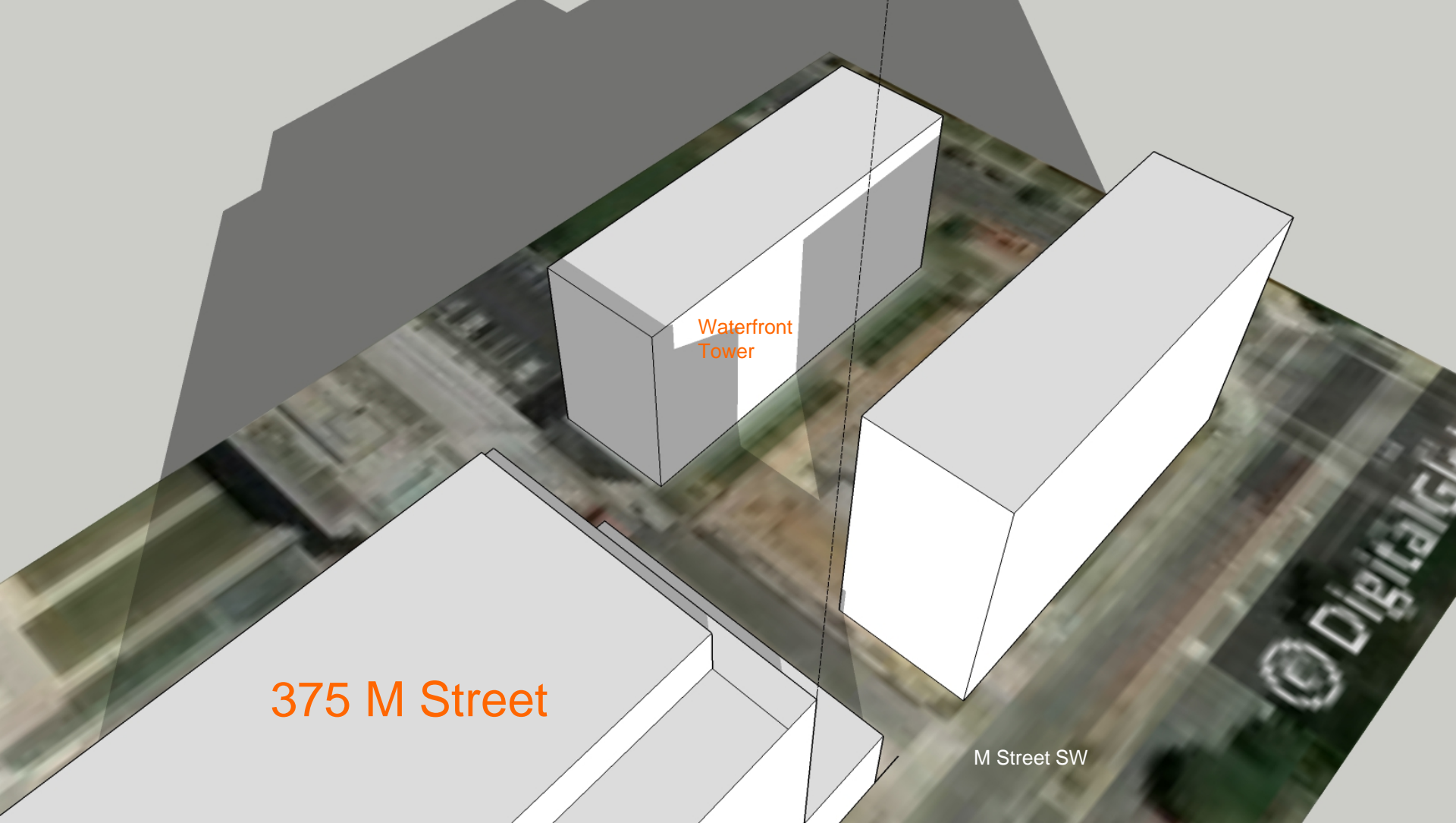
12 Story Building (as proposed), 15' Setback (as requested for streetscape) 3.00pm 21 December Winter Solstice
